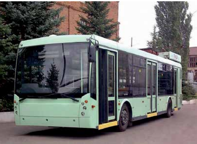
The ECObus-5250 operates entirely with batteries charged by an onboard Capstone C65 Microturbine.
